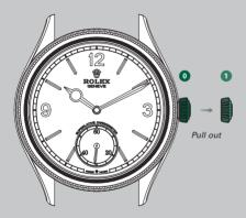
After every use, return the crown to *position 0*. The crown should never be adjusted underwater.
