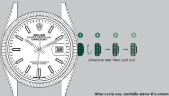
After every use, carefully screw the crown back down against the case to guarantee the waterproofness. Return the crown to position 1 and apply light pressure on it while screwing it down clockwise against the case. The crown should never be unscrewed underwater.
