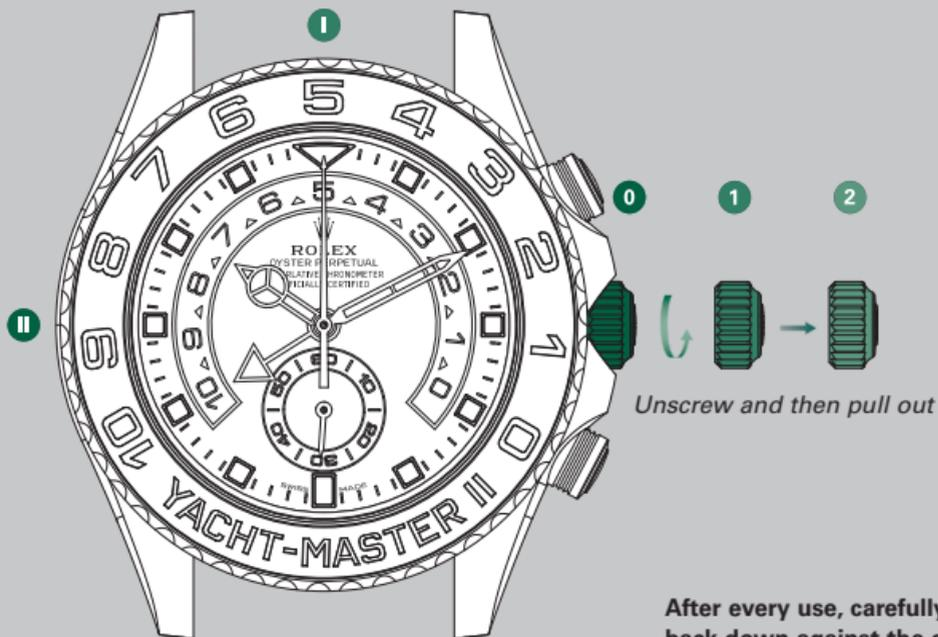
After every use, carefully screw the crown back down against the case to guarantee the waterproofness. Return the crown to *position 1* and apply light pressure on it while screwing it down clockwise against the case. The crown should never be unscrewed underwater.
