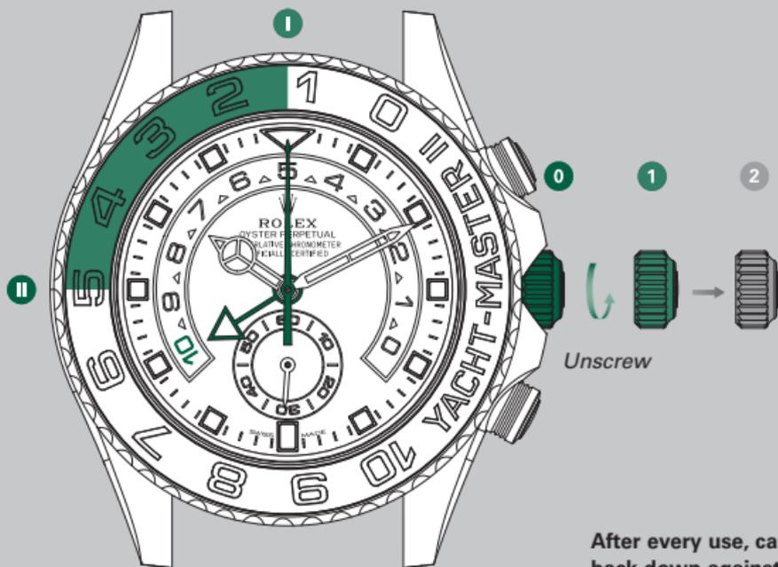
After every use, carefully screw the crown back down against the case to guarantee the waterproofness. Return the crown to *position 1* and apply light pressure on it while screwing it down clockwise against the case. The crown should never be unscrewed underwater.
