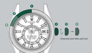
waterproofness. Return the crown to position 1 and apply light pressure on it while screwing it down clockwise against the case. The crown \* The date shown here is 28 August should never be unscrewed underwater.
