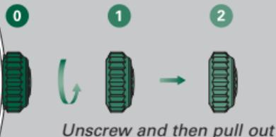
After every use, carefully screw the crown back down against the case to guarantee the waterproofness. Return the crown to *position 1* and apply light pressure on it while screwing it down clockwise against the case. The crown should never be unscrewed underwater.
