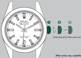
After every use, carefully screw the crown back down against the case to guarantee the waterproofness. Return the crown to *position 1* and apply light pressure on it while screwing it down clockwise against the case. The crown should never be unscrewed underwater. ROLEX SERVICE
