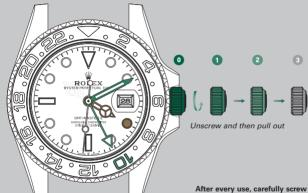
\* Reference time, Geneva, 10.10 a.m. \* Local time, New York, 4.10 a.m. After every use, carefully screw the crown back down against the case to guarantee the waterproofness. Return the crown to *position 1* and apply light pressure on it while screwing it down clockwise against the case. The crown should never be unscrewed underwater. USING YOUR WATCH ROLEX SERVICE
