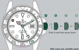
\* Reference time, Geneva, 10.10 a.m. \* Local time, Geneva, 10.10 a.m. After every use, carefully screw the crown back down against the case to guarantee the waterproofness. Return the crown to *position 1* and apply light pressure on it while screwing it down clockwise against the case. The crown should never be unscrewed underwater.
