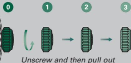
After every use, carefully screw the crown back down against the case to guarantee the waterproofness. Return the crown to *position 1* and apply light pressure on it while screwing it down clockwise against the case. The crown should never be unscrewed underwater.
