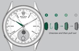
After every use, carefully screw the crown back down against the case to guarantee the waterproofness. Return the crown to *position* 1 and apply light pressure on it while screwing it down clockwise against the case. The crown should never be unscrewed underwater. USING YOUR WATCH ROLEX SERVICE
