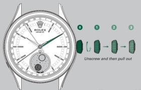
After every use, carefully screw the crown back down against the case to guarantee the waterproofness. Return the crown to position 1 and apply light pressure on it while screwing it down clockwise against the case. The crown should never be unscrewed underwater.
